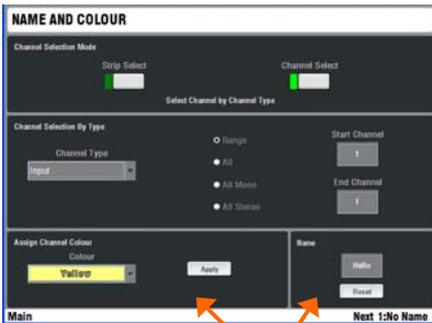
**Strip Select / Single Strip Select** - Press a strip **SEL** key. Touch Name to open the on-screen keypad. Touch Colour to select a colour. Touch Apply.
